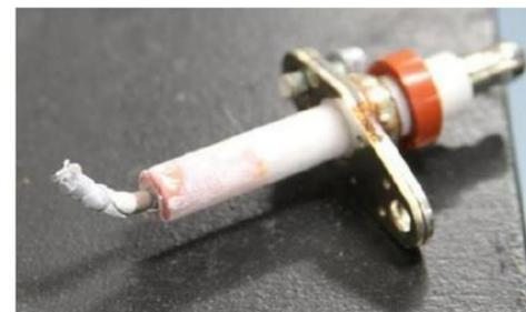
Figure 26: Ionization probe from boiler 1 covered with silica.
